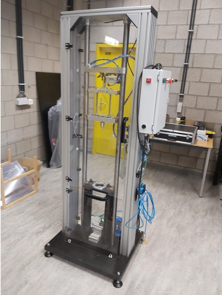
Figure 8.3: Picture of the as built impact tower with the controller in the white box on the right side, adjustable weights and sample holder in the middle between two finely machined rods used to guide the falling weights
