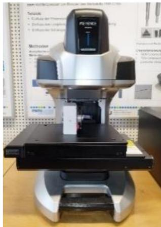
**Figure 2-9** Keyence optical measuring machine
