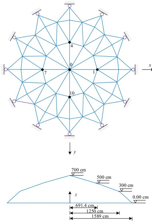
Fig. 12. A 120-bar space truss structure for Example 4.
