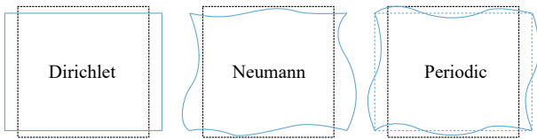
Figure 5: Deformation of body B for different boundary conditions.
